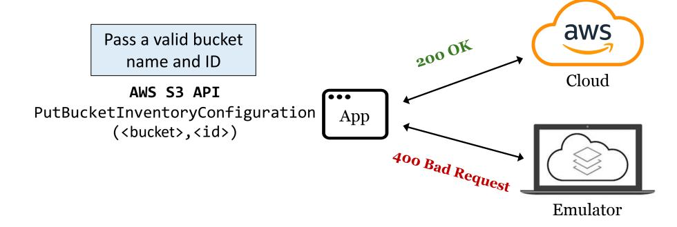
Emulator inaccurately simulates S3's regional access causing error response to a valid request
